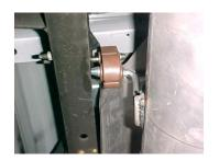
Install welded muffler hanger into rubber grommets.
