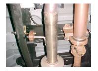
Install welded headpipe hanger into rubber grommet.
