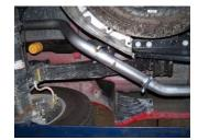
**5.** Install the passenger side overaxle tailpipe #C into the muffler 1½"-2". Use clamp #H to secure tailpipe to muffler. DO NOT TIGHTEN. Insert hanger into rubber grommet.
