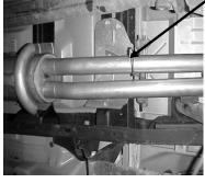
INTSTALL EXIT PIPES # F TO THE OVERAXLE TAILPIPES USE CLAMP # G TO SECURE USE ZIP TIES FOR BRAKE AND HOSE LINES TO KEEP AWAY FROM PIPES. NOW FIRMLY TIGHTEN ALL BOLTS, CLAMPS AND HANGERS. INSTALL STAINLESS TIPS.
