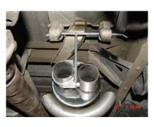
INSTALL MUFFLER #B ONTO HEADPIPE 1-1/2" TO 2". OUTLET SHOULD BE LEVEL. USE CLAMP #J TO SECURE MUFFLER TO HEADPIPE. DO NOT TIGHTEN. INSTALL REAR MUFFLER HANGER #G ONTO THE DRIVERSIDE MUFFLER OUTLET. INSERT HANGERS INTO RUBBER GROMMETS. DO NOT TIGHTEN.
