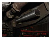
INSTALL HEADPIPE #A ONTO FACTORY PIPE USING CLAMP #K TO SECURE TOGETHER. DO NOT TIGHTEN.
