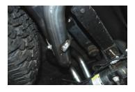
INSTALL PASS. SIDE TAILPIPE # C INTO MUFFLER 1 1 TO 2". INSERT HANGER INTO RUBBER GROMMET. USE CLAMP # G TO SECURE PIPE TO MUFFLER, DO NOT TIGHTEN.
