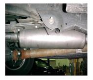
INSTALL MUFFLER # B ONTO HEADPIPE 1 1 TO 2". USE CLAMP # F TO SECURE MUFFLER TO HEADPIPE. DO NOT TIGHTEN. USE A JACK STAND TO HOLD UP THE MUFFLER. OUTLETS SHOULD BE LEVEL.
