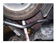
**6.** Install the driverside overaxle tailpipe #D into the muffler 1<sup>1</sup>/<sub>2</sub>-2". Use clamp #H to secure. DO NOT TIGHTEN. Rotate until it meets with the rubber grommet, use clamp #H to hold pipe. DO NOT TIGHTEN.
