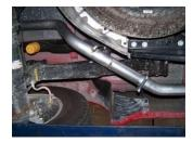
**4.** Install the passenger side overaxle tailpipe #C into the muffler 1½"-2". Use clamp #H to secure tailpipe to muffler. DO NOT TIGHTEN. Insert hanger into rubber grommet.
