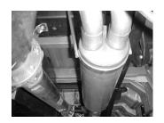
SLIP MUFFLER #B THROUGH BAND CLAMP THEN ONTO THE HEADPIPE 1 ½" TO 2". THE OUTLETS WILL BE LEVEL. USE CLAMP #G TO SECURE MUFFLER TO HEADPIPE. DO NOT TIGHTEN.
