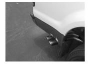
INSTALL YOUR STAINLESS TIPS. TIGHTEN ALL CLAMPS STARTING FROM THE FRONT, WORKING YOUR WAY TO THE BACK OF THE TRUCK. TO CLEAN TIPS USE A STAINLESS STEEL CLEANER & SCOTCH BTIE PAD.
