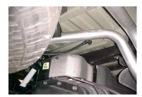
INSTALL DRIVERS SIDE TAILPIPE # D INTO MUFFLER 1 ½" TO 2". INSERT WELDED HANGERS INTO RUBBER GROMMETS. USE CLAMP # H TO SECURE PIPE TO MUFFLER, DO NOT TIGHTEN.
