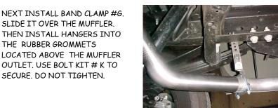
INSTALL PASSENGER SIDE OVERAXLE PIPE #C INTO **MUFLER** 1 ½" TO 2". USE CLAMP # I TO
