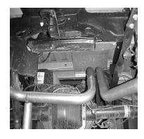
THE SPARE TIRE MAY NEED TO BE LOOSENED AND PUSH TO THE DRIVER SIDE AND THEN ROTATE THE OVERAXLE PIPE TO GAIN CLEARANCE.
