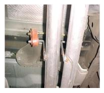
INSTALL THE DRIVERSIDE FRONT TAILPIPE # D TO **OUTLET OF MUFFLER** 1.5" TO 2". THE TAILPIPE INLET THAT GOES INTO THE MUFFLER IS 4.5" LONG. **INSERT HANGER INTO** RUBBER GROMMET. ATTACH WITH HANGER# G. INSTALL DRIVERSIDE OVERAXLE TAILPIPE # E TO FRONT DRIVERSIDE TAILPIPE, THIS PART HAS A SWEDGE UP ON IT. ATTACH USING CLAMP
