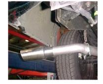
EXIT PIPE, THEN INTSTALL EXIT PIPES # F TO THE **OVERAXLE** TAILPIPES, USE CLAMP #G TO SECURE. USE ZIP TIES FOR BRAKE AND HOSE LINES TO KEEP AWAY FROM PIPES. NOW FIRMLY TIGHTEN ALL BOLTS, CLAMPS AND HANGERS. **INSTALL YOUR STAINLESS** TIPS TO YOUR DESIRED LOOK.
