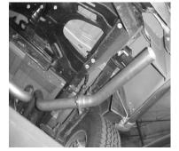
**INSTALL PASSENGER** OVERAXLE TAILPIPE TO THE **OUTLET OF THE MUFFLER** 1.5" TO 2". THE TAILPIPE INLET THAT GOES INTO THE MUFFLER IS 4.5" LONG AND ATTACH WITH CLAMP # G. DO NOT TIGHTEN. INSERT WELDED HANGER INTO RUBBER GROMMET.
