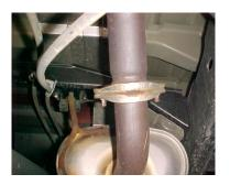
LAY OUT THE GIBSON EXHAUST ON THE FLOOR AND COMPARE PART #'S TO THE DRAWING. TO REMOVE YOUR FACTORY EXHAUST UN-BOLT YOUR TAILPIPE AT THE 2-BOLT FLANGE LOCATED BEHIND YOUR STOCK MUFFLER USE WD-40 TO AID YOU IN REMOVAL OF HANGERS FROM RUBBER GROMMETS.
