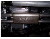
4. Install muffler #C onto headpipes 1.5"-2" with the louvers facing towards the converter. Use a jack stand to support the muffler. Use clamps #J to secure the muffler to the headpipes. Do not tighten. Muffler inlet is looking into the louvers.
