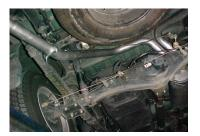
INSTALL THE DRIVERSIDE OVER AXLE TAILPIPE #C ONTO MUFFLER 1-1/2" TO 2" USE CLAMP # I TO SECURE PIPE TO MUFFLER, DO NOT TIGHTEN.
