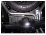
8. Install driver side overaxle tailpipe #G onto extension pipe, use clamp #J to secure pipe. Do not tighten. Insert welded hanger into rubber grommet.
