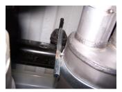
**3.** Install muffler #B onto head pipe #A  $1\frac{1}{2}$ "-2" with the louvers facing towards the converter. Use a jack stand to support the muffler. Use clamp #H to secure the muffler to the headpipe. Slide band clamp #I onto muffler and insert welded hangers into rubber grommets. Attach with bolt kit #K. DO NOT TIGHTEN. Muffler inlet is looking into the louvers.
