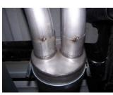
6. Install driver side tailpipe #D  $1\frac{1}{2}-2$ " into muffler and use clamp #G to secure to muffler. Attach clamp #G to hold up to the hanger **#F. DO NOT TIGHTEN.**
