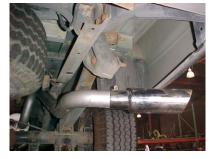
MAKE SURE YOU HAVE A MIMIMUM OF AT LEAST 1" OF CLEARANCE FROM ALL BRAKE LINES, SHOCKS, TIRES, ETC. SPARE TIRE MAY NEED TO BE LOOSENED AND PUSHED TO THE REAR OF THE TRUCK FOR BETTER CLEARANCE.
