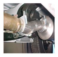
INSTALL HEADPIPE #A, YOU WILL NEED TO LINE UP THE TWO NOTCHES. INSERT HANGER INTO RUBBER GROMMET. DO NOT TIGHTEN. USE CLAMP #M TO SECURE HEADPIPE TO YOUR STOCK PIPE.
