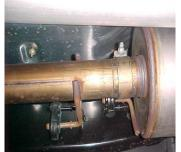
YOU MAY NEED TO HEAT IT UP FOR EASIER REMOVAL. LEAVE ALL RUBBER GROMMETS IN PLACE. USE WD-40 FOR REMOVAL OF HANGERS.
