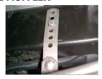
MEASURE 19 ½" FROM THE REAR OF THE FRAME AND USE THIS HOLE AND BOLT ON HANGER #F. USE THE 3<sup>RD</sup> HOLE FROM THE TOP.
