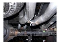
**INSTALL PASSENGER** SIDE TAILPIPE #D INTO MUFFLER AND ATTACH USING CLAMP #F. **INSERT WELDED** HANGER INTO RUBBER GROMMET. DO NOT TIGHTEN. USE BOLT KIT #I TO ATTACH THE TAILPIPES TOGETHER. DO NOT TIGHTEN. PASSENGER SIDE TABS ON TAILPIPE WILL BE ON TOP OF DRIVER SIDE TABS. YOU MAY NEED TO LOOSEN THE SPARE TIRE AND PUSH TOWARD THE DRIVERSIDE FOR EASIER INSTALLATION.
