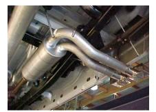
**INSTALL MUFFLER** ASSEMBLY #A ONTO HEADPIPE 1-1/2" TO 2". SLIDE WELDED HANGERS INTO RUBBER GROMMETS YOU MAY NEED TO ADJUST WELDED HANGERS TO FIT INTO YOUR GROMMETS. USE A JACKSTAND TO SUPPORT YOUR MUFFLER. USE CLAMP #B TO SECURE IT TO YOUR HEADPIPE. DO NOT TIGHTEN.
