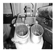
CONNECT MUFFLER #B WITH INLET TOWARDS THE CONVERTER TO THE HEADPIPE. ATTACH TO HEADPIPE WITH CLAMP #J. USE A JACK STAND TO SUPPORT THE MUFFLER. INSTALL HANGER #H AT THE REAR OF THE MUFFLER ON THE DRIVER SIDE OUTLET AND INSERT WELDED HANGER INTO RUBBER GROMMET. (MAKE SURE OUTLETS OF MUFFLER ARE LEVEL AND HANGER #H IS POSITIONED.
