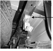
INSTALL HANGERS #G TO BOTTOM OF FRAME RAIL IN EXISTING HOLE APPROXIMATELY 19 1/4" FROM REAR OF FRAME. USE NUT AND BOLT SUPPLIED.
