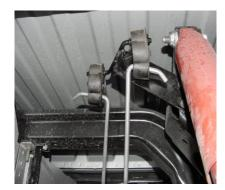
INSTALL MUFFLER ASSEMBLY #B ONTO HEADPIPE 1-1/2" TO 2". SLIDE WELDED HANGERS INTO RUBBER GROMMETS YOU MAY NEED TO ADJUST WELDED HANGERS TO FIT INTO YOUR GROMMETS. USE A JACKSTAND TO SUPPORT YOUR MUFFLER. USE CLAMP #C TO SECURE IT TO YOUR HEADPIPE. DO NOT TIGHTEN.
