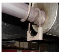
TO REMOVE STOCK EXHAUST UNCLAMP IT FROM THE CLAMP LOCATED JUST IN FRONT OF YOUR STOCK MUFFLER. YOU MAY NEED TO HEAT IT UP WITH A TORCH TO REMOVE IT. NOW CUT OFF YOUR STOCK TAILPIPE JUST BEHIND THE MUFFLER AND REMOVE.LEAVE ALL RUBBER GROMMETS ON THE HANGER. USE WD-40 TO AID IN REMOVAL OF EXHAUST AND HANGERS.
