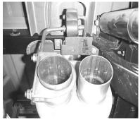
INSTALL REAR MUFFLER HANGER #F ON THE DRIVERSIDE OUTLET AND INSERT INTO RUBBER HANGER.MAKE SURE OUTLETS OF MUFFLER ARE LEVEL AND HANGER #F IS POSITIONED CORRECTLY.
