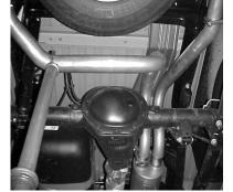
INSTALL PASSENGER SIDE OVERAXLE PIPE #D AND ATTACH TO MUFFLER USING CLAMP # F. ATTACH HANGER # H AND CLAMP #F TO OVERAXLE TAILPIPE.
