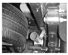
1. TO REMOVE YOUR EXHAUST 2WD- CUT 8" IN FRONT OF YOUR STOCK MUFFLER.
