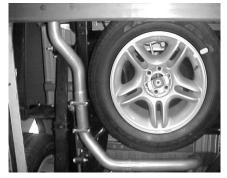
4. INSTALL DRIVERSIDE TAILPIPE PIPE # C INTO MUFFLER AT LEAST 1  $\frac{1}{2}$ " NO MORE THAN 2". ATTACH TAILPIPE TO MUFFLER WITH CLAMP # G, AND ATTACH HANGERS # I TO TAILPIPES.NEXT INSTALL OVERAXLE PIPE #E TO FRONT TAILPIPE, USE CLAMP # G TO SECURE PIPES. DO NOT TIGHTEN YET.
