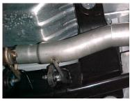
INSTALL HEADPIPE #A, YOU WILL NEED TO LINE UP THE TWO NOTCHES. INSERT WELDED HANGER INTO RUBBER GROMMET. USE CLAMP #G TO SECURE HEADPIPE TO THE STOCK PIPE. DO NOT TIGHTEN.
