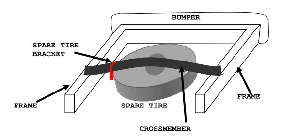
THIS SPARE BRACKET IS USED FOR BETTER CLEARANCE FROM THE SPARE TIRE. INSTALL THIS BRACKET ON THE FACTORY CROSS MEMBER LOCATED ABOVE THE SPARE TIRE. THIS BRACKET IS DESIGNED TO HOLD THE SPARE TIRE TOWARDS THE DRIVERSIDE GIVING YOU MORE CLEARANCE ON THE TAILPIPES.
