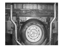
INSTALL PASSENGER SIDE OVERAXLE TAILPIPE # C 1-1/2" TO 2" FROM BEHIND THE AXLE AND CONNECT TO THE MUFFLER AND ATTACH WITH CLAMP #F. INSERT WELDED HANGER INTO RUBBER GROMMET. ATTACH HANGER #H USING CLAMP #F TO TAILPIPE.
