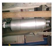
INSTALL MUFFLER AND ATTACH TO HEADPIPE. USING CLAMP #G. DO NOT TIGHTEN. USE JACKSTAND TO SUPPORT MUFFLER.
