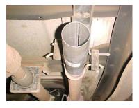
INSTALL HEADPIPE # A AND ATTACH TO THE STOCK EXTENSION PIPE USING CLAMP #F
