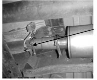
DO NOT REMOVE THE STOCK EXTENSION PIPE BETWEEN THE CONVERTER AND MUFFLER. UNCLAMP EXHAUST IN FRONT OF THE STOCK MUFFLER JUST BEFORE THE STOCK RUBBER HANGER. CUT THE STOCK OVERAXLE PIPE JUST AFTER THE MUFFLER WITH A HACKSAW. LEAVE ALL RUBBER GROMMETS ON. APPLY WD-40 TO ALL HANGERS FOR EASIER REMOVAL.
