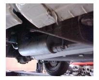
Install the driver side over axle tailpipe # D into the muffler. Use clamp # F to secure tailpipe to muffler. Do not tighten. Insert hanger into rubber grommet.
