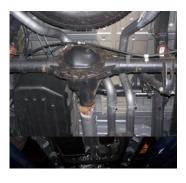
7. Install passenger side tailpipe #C into muffler at least 1.5" to 2". Use clamp #G to secure pipe to muffler. Do not tighten. The tailpipes will both lean towards the driver side for clearance. Insert welded hangers into rubber grommets.
