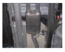
4. Install muffler #B with inlet towards Y-pipe. Use jack stands to support the muffler. Use clamp #F to secure the muffler to headpipe. Do not tighten.
