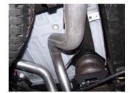
5. Slide the over axle tailpipe #C into the muffler 1.5-2". Use clamp #E to secure tailpipe to muffler. Do not tighten. Insert welded hangers into rubber grommets.
