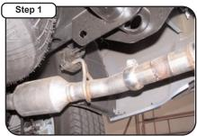
To remove the stock exhaust, remove your factory exit pipes. Next, remove your tailpipes by unbolting them from the back of your stock muffler. Remove your factory muffler from the clamp in front of it. Use WD-40 to aid in removal of factory grommet that will be re-used.
