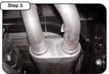
Install muffler #B onto head pipe #A 1 1/2"-2". Use a jack stand to support the muffler. Use clamp #G to secure the muffler to the head pipe. Do not tighten.
