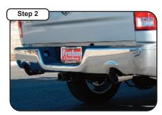
Attach Stainless Steel Tips. When you have everything in place, firmly tighten all bolts and clamps down securely. Use stainless steel cleaner and a Scotch Brite pad weekly to prevent tip from discoloration. Inspect all fasteners after 25-50 miles of operation and re-tighten if necessary.
