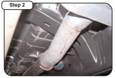
Install head pipe # A onto your existing stock front pipe and attach with clamp #G. Do not tighten . Insert welded hanger into rubber grommet.
