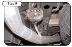
Install drivers side overaxle tailpipe #D into the muffler. Use clamp #H to secure. Do not tighten. Insert welded hangers into rubber grommets.
