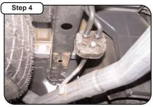
Install the passenger side overaxle tailpipe # C to the muffler 1 1/2"-2". Use clamp #H to secure tailpipe to muffler. Do not tighten. Insert welded hangers into rubber grommets.
