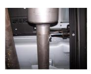
4. Slide muffler #B over headpipe 1.5-2" with the louvers facing towards the converter. Use a jack stand to support the muffler. Use clamp #E to secure the muffler to the headpipe. Do not tighten. Muffler inlet is looking into the louvers.
