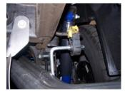
**5.** Install Passenger side tailpipe #D into muffler outlet 1½-2". Insert welded hangers into rubber grommet. Use clamp #F to attach to tailpipe to muffler. DO NOT TIGHTEN.
