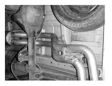
Install the Passenger side over-axle tailpipe # D to the muffler, 1-1/2" to 2". Use clamp # G to secure the tailpipe to the muffler. Use Bolt kit #I to attach the tailpipes together. **Do not Tighten at this Time!** Driver side tab will be on the bottom.
