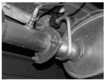
Lay out the exhaust on the floor so it looks like the drawing and compare the parts with the manual. To remove the stock exhaust, un-bolt it from the 3-bolt flange located in front of the muffler. NOTE: For an easy removal of the exhaust, cut the tailpipe off behind the muffler. Leave all rubber grommets in place. Use WD-40 to aid in removal.
