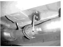
Install your head-pipe # A onto your existing stock flange, use your supplied hardware #J & K in the kit. Use a jack stand to support the converter. Insert the welded hanger into the rubber grommet.
