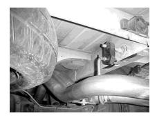
Install the Driver side over-axle tailpipe #C into the muffler 1-1/2" to 2". Then insert the welded hanger into the rubber grommet. Use clamp #H to secure it to the muffler. **Do Not Tighten at this Time!**
