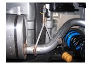
2. To remove the stock exhaust, remove it from the two bolt flange in front of the muffler. Do not remove, you will re-use bolts. Disengage the welded hangers using WD-40 from the OEM rubber grommets. Do not damage or remove the rubber grommets as you will reuse them to mount your new system. Now, cut off tailpipe before and after rear axle for removal.
