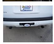
**8.** Install the exit pipes #E. Use clamp #G to secure exit pipes to tailpipes. DO NOT TIGHTEN. Rotate pipes to adjust for desired look. Reinstall spare tire.
