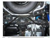
**7.** Install driver side tailpipe #C into the muffler 1½-2". Use clamp #G to secure tailpipe to muffler. DO NOT TIGHTEN. Insert welded hangers into rubber grommets.
