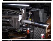
**8.** Install the exit pipes #E. Use clamp #G to secure exit pipes to tailpipes. DO NOT TIGHTEN. Reinstall spare tire. Use zip ties to secure brake, gas lines as necessary.
