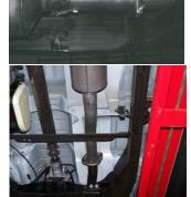
**5.** Install passenger side tailpipe #D to the muffler 1½-2". Use clamp #G to secure tailpipe to muffler. DO NOT TIGHTEN. Insert welded hangers into rubber grommet.
