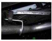
**9.** Install the exit pipes #E and #F. Use clamp #H to secure exit pipes to tailpipes. DO NOT TIGHTEN.
