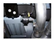
8. Install driver side tailpipe #C to the muffler 1½-2". Use clamp #H to secure tailpipe to muffler. DO NOT TIGHTEN. Insert welded hangers into rubber grommets.
