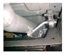
INSTALL HEAD PIPE # A ONTO YOUR EXISTING STOCK FRONT PIPE. INSERT WELDED HANGER INTO RUBBER GROMMET.
