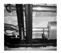
LAY OUT THE GIBSON EXHAUST ON THE FLOOR AND COMPARE PART #'S TO THE DRAWING. TO REMOVE STOCK EXHAUST, REMOVE IT FROM THE 2-BOLT FLANGE LOCATED IN FRONT OF THE MUFFLER. DO NOT DISGUARD FACTORY HARDWARE YOU WILL RE-USE IT. LEAVE ALL RUBBER GROMMETS IN PLACE. USE WD-40 TO AID IN REMOVAL OF EXHAUST AND THE RUBBER GROMMETS.
