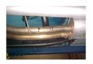
Lay out the exhaust on the floor so it looks like the drawing and compare parts with manual. To remove the stock exhaust cut 13" just in front of the muffler.
