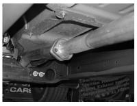
BOLT HEADPIPE #A TO STOCK FLANGE RE-USING FACTORY NUTS. DO NOT TIGHTEN. SLIDE WELDED HANGER INTO RUBBER GROMMET
