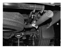
INSTALL PASSENGER SIDE TAILPIPE #C INTO MUFFLER AT LEAST 1  $\frac{1}{2}$ " TO 2". USE CLAMP #G TO SECURE PIPE TO MUFFLER. DO NOT TIGHTEN. THE TAILPIPES WILL BOTH LEAN TOWARDS THE DRIVER SIDE FOR CLEARANCE.
