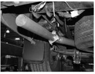
INSTALL DRIVER SIDE TAILPIPE #D INTO MUFFLER AT LEAST 1  $\frac{1}{2}$ " TO 2". THIS PIPE WILL ROUTE OVER THE AXLE AND BETWEEN THE SHOCK AND TIRE. ATTACH CLAMP #I TO SECURE TAILPIPE TO MUFFLER. DO NOT TIGHTEN. LOOKING FROM THE REAR OF THE VEHICLE - THIS TAILPIPE IS AT APPX. 11 O'CLOCK.
