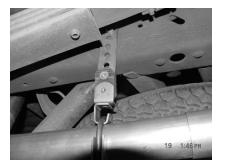
REMOVE STOCK REAR HANGER FROM FRAME ON PASSENGER SIDE. INSTALL 10" METAL HANGER #H. USE THE FIFTH HOLE FROM THE BOTTOM. INSTALL IT IN THE FACTORY HOLE WHERE THE STOCK HANGER WAS IN. IT IS LOCATED APPROX. 20" FROM REAR OF FRAME 3/8" HOLE.
