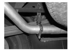
INSTALL EXIT PIPES #E ONTO TAILPIPES. ROLL EXIT PIPES UNTIL YOU HAVE THE CORRECT ANGLE. USE CLAMPS #G TO SECURE TO THE TAILPIPES. DO NOT TIGHTEN. CUT EXIT PIPE TO PROPER LENGTH.
