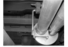
UNBOLT THE 2-BOLT FLANGE LOCATED BEHIND THE CONVERTER, SAVE STOCK NUTS AND BOLTS FOR YOU WILL REUSE THEM. NOW CUT OFF YOUR STOCK TAILPIPE JUST BEHIND THE MUFFLER AND REMOVE. USE WD-40 TO AID IN REMOVAL OF THE EXHAUST AND HANGERS. LEAVE ALL RUBBER GROMMETS ON THE HANGER.
