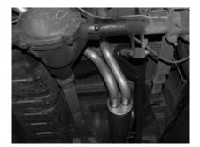
INSTALL PASSENGER SIDE TAILPIPE #C INTO MUFFLER 1-1/2" TO 2" USING CLAMP #G THIS WILL HOLD UP THE PIPE. ATTACH CLAMP #G TO TAILPIPE AND SECURE WITH HANGER #H. DO NOT TIGHTEN.
