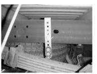
Remove the stock rear hanger from frame on passenger side. Install hangers # H to the frame using existing bottom hole where the stock hanger was mounted. Use the supplied nuts and bolts and mount the hanger through the fifth hole down from the top of the hanger. Repeat on the driver side.
