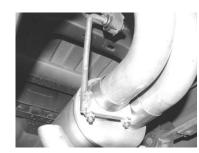
Install hanger #I onto the rear outlet of the muffler on the driver side. Insert the vertical rod through the rubber grommet from the driver side towards the passenger side. Do not tighten.
