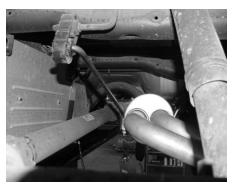
INSTALL HANGER #F INTO RUBBER GROMMET LOCATED JUST ABOVE TAILPIPE ASSEMBLY, SLIDE CLAMP THAT IS WELDED TO THE HANGER OVER DRIVERSIDE TAILPIPE. DO NOT TIGHTEN.
