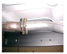
TO REMOVE STOCK EXHAUST UN-BOLT IT FROM THE 2-BOLT FLANGE LOCATED JUST BEHIND THE Y-PIPE. **DO NOT DAMAGE FACTORY HARDWARE, YOU WILL RE-USE IT.** NOW CUT OFF YOUR STOCK TAILPIPE JUST BEHIND THE MUFFLER AND REMOVE. LEAVE ALL RUBBER GROMMETS ON THE HANGER. USE WD-40 TO AID IN REMOVAL OF EXHAUST AND HANGERS.
