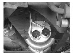
Install muffler with the inlet towards the converter onto the head pipe at least 1-1/2" to 2" using clamp # G. Use a jackstand to support. The inlet of the muffler should be at about 6'oclock.Do not tighten.
