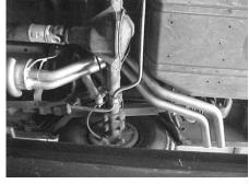
Install the passenger side over axle tailpipe #C onto muffler at least 1-1/2" to 2" using clamp #F to attach tailpipe. Do not tighten. Install Driver side over axle tailpipe #D onto Muffler at least 1-1/2" to 2" using hanger #H to attach tailpipe. Insert into rubber grommet. Use Bolt Kit #I to secure both tailpipes together.
