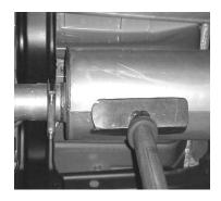
INSTALL MUFFLER # B ONTO HEADPIPE #A 1 1/2" TO 2"". THE INLET WILL BE AT **APPROXIMATELY** 6 O'CLOCK, CONNECT THE MUFFLER TO HEADPIPE#A USING CLAMP#F. INSERT WELDED HANGER INTO RUBBER GROMMET.
