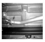
BOLT HEADPIPE # A TO YOUR STOCK FLANGE RE-USING FACTORY BOLTS. AND NUTS. DO NOT TIGHTEN INSERT WELDED HANGER INTO RUBBER GROMMET.
