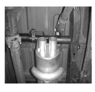
INSTALL MUFFLER # B WITH INLET TOWARDS Y-PIPE, WITH THE OUTLETS POSITIONED AT THE TOP OF THE MUFFLER. USE A JACK STAND TO SUPPORT THE MUFFLER. USE CLAMP #F TO CONNECT THE MUFFLER TO HEADPIPE. INSTALL HANGER # H ONTO THE DRIVERSIDE OUTLET OF THE MUFFLER. INSERT THE WELDED HANGER INTO THE RUBBER GROMMET FROM THE PASSENGER SIDE. DO NOT TIGHTEN.
